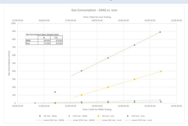
**I-CO<sub>2</sub>N<sub>2</sub>IC Gas Consumption Test.** The results of a steady-state test (InvivO<sub>2</sub> 400 set to 0.1% O<sub>2</sub> and 0.5% CO<sub>3</sub>). ICO<sub>3</sub>N<sub>2</sub>IC used 296 L of N<sub>3</sub> over the test period, a reduction of 40% over the previous technology.
